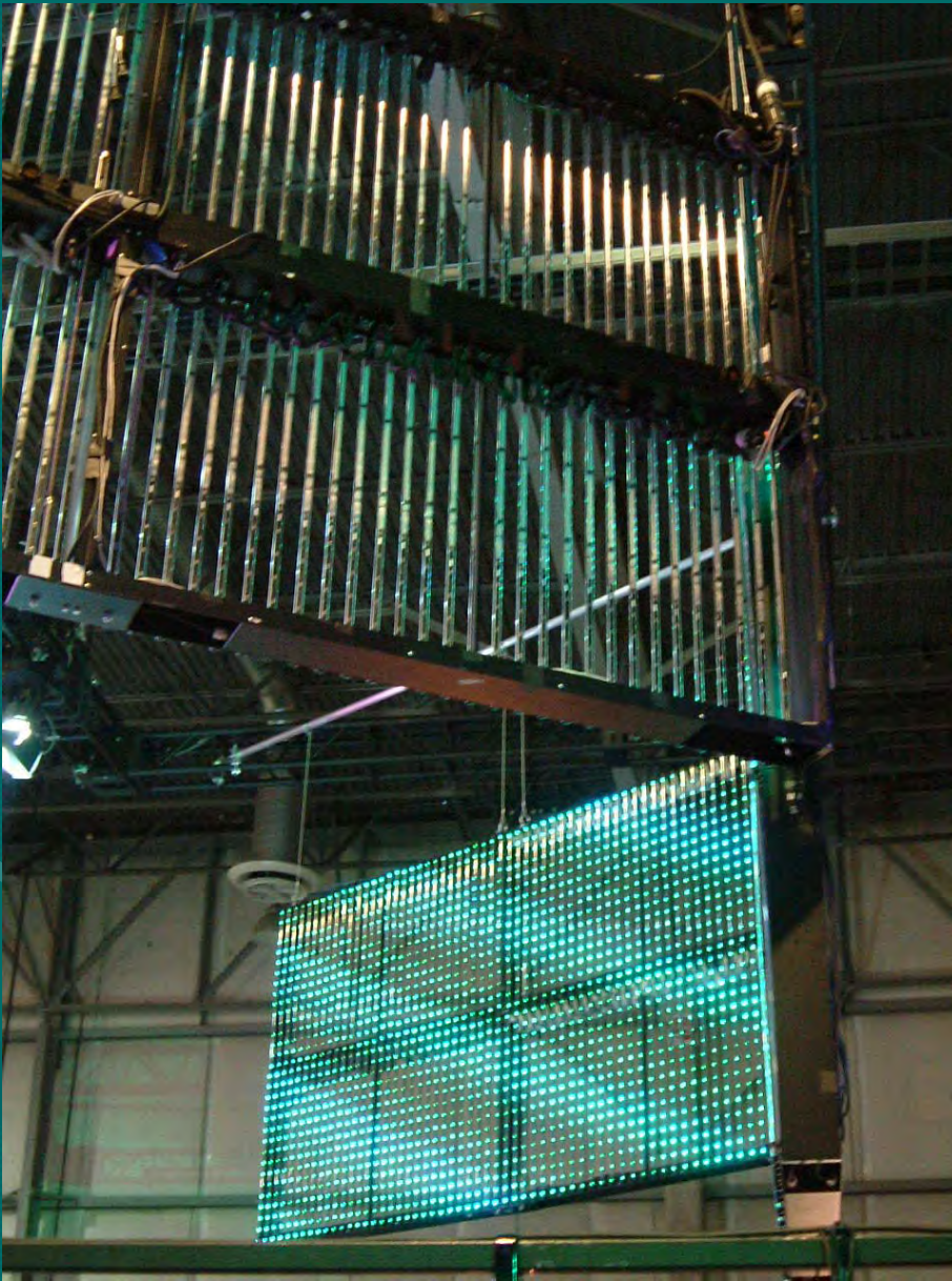
Translucent display using LED lamps
